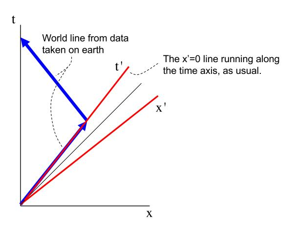
As usual, lines of simultaneity in the primed axis system will be parallel to the x' axis (the lines of simultaneity for the take-off point and for the turn-around point are shown below).
